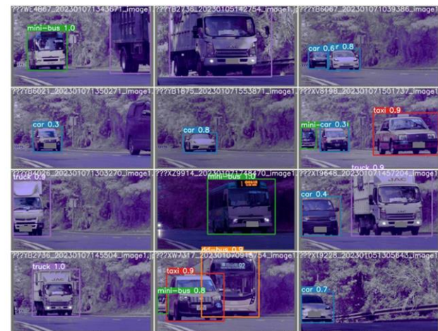
Examples of the output from the customized YOLOv8 model, with the confidence value as marked at the top of each detected vehicle
