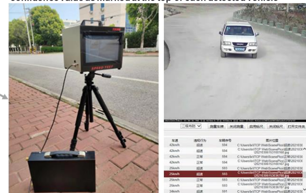
Photo of the plate number camera and the user's interface
