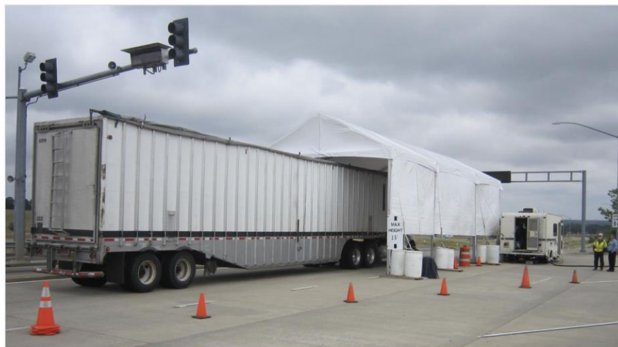
Heavy-duty diesel truck entering the plume capture facility.
