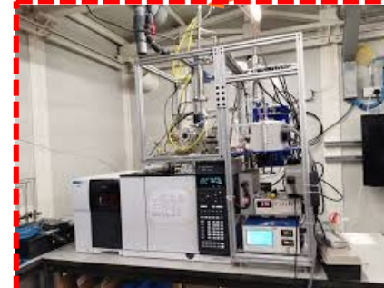
Thermal desorption Aerosol Gas Chromatography-Mass Spectrometry analyzer (TAG-GCMS)
